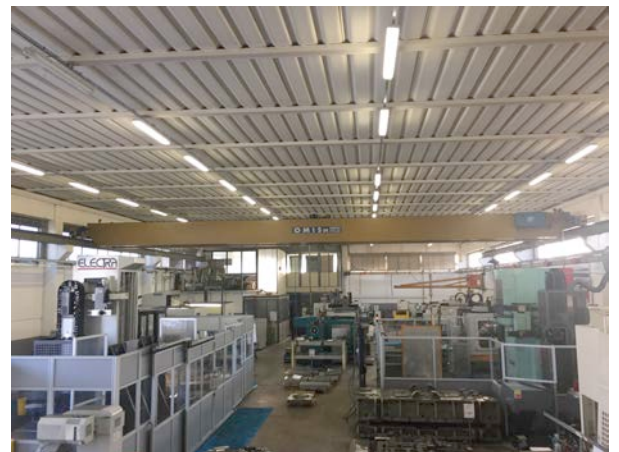
Nr° 2 Carri ponte da 15 Ton. Nr° 2 Overhead travelling cranes from 15 Tons.
